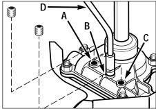
Figure 14: Transmission lubricant check and fill locations.
